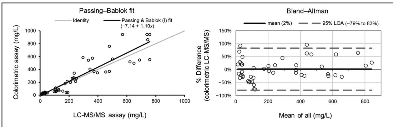
**Fig. 5. Comparison (n = 47) of cystine measurement by colorimetric and LC-MS/MS assays.**
