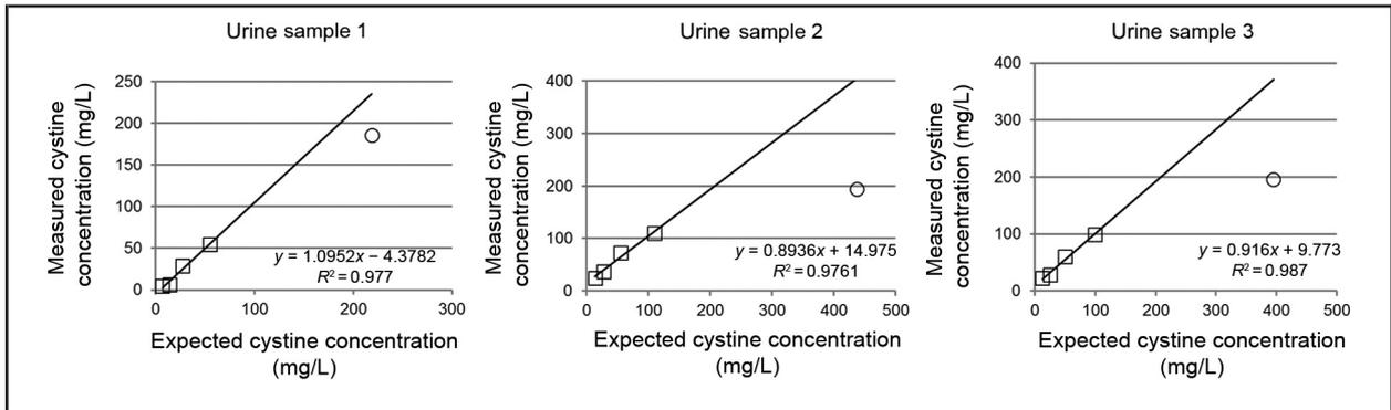
**Fig. 4. Linearity of cystine measurement in spiked urine.**
